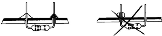
Trim excess leads as close as possible to the solder joint
