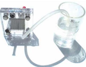
**Step 9:** Place the Oxygen tank (E) next to the reversible fuel cell (C) on the same side as the red hose pin and red banana socket. Attach the 16cm rubber hose (G) from the gas container (F) inside the Oxygen tank (D) to the lower right nozzle on the same side as the red hose pin and the red banana socket.
