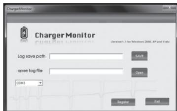
The COM port to be used can be found in the Windows Control Panel (in the Device Manager, under "COM & LPT"). Usually, it is "COM3".
