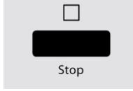
Press the **Stop** button for three seconds until a signal tone is heard and the illumination on the function display goes out. In the locked state, all the buttons are disabled.
