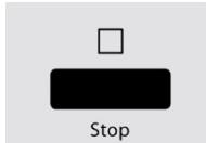
Press the **Stop** button for three seconds until a signal tone is heard and the function display lights up. In the locked state, all the buttons are disabled.
