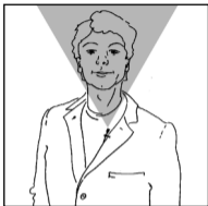
Fig. 4: Microphone pickup angle.
