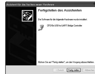
Fig. 12: Successful installation of the second driver
