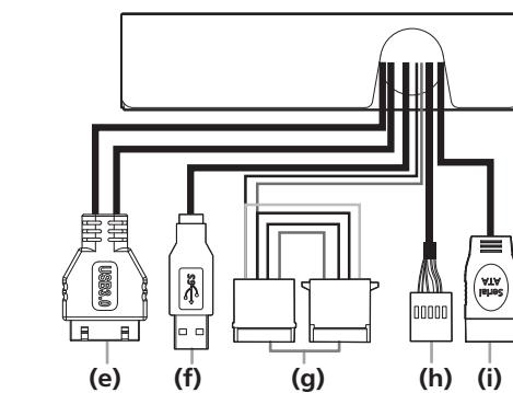
**GB** **(e)** internal motherboard USB 3.0 connector **(f)** USB 3.0 A male connector **(g)** 4-Pin PSU molex connector
