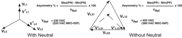
The voltage asymmetry causes the rise in motor temperature and a reduction of the rated motor power. Voltage asymmetry limit values can be adjusted between 5%-15% by the user or can be disabled. Hysteresis is 30% of the adjusted asymmetry value. Example: Given 3x380 V supply with 10% asymmetry, Relay switches OFF at:  $380 \cdot (10 \cdot 400 / 100) = 340 \text{ V}$  Relay switches ON at:  $380 \cdot ((10 - (10 \cdot 30)) \cdot 400 / 100) = 353,2 \text{ V}$
