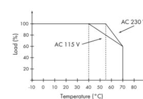
Fig. 5: Derating curve
