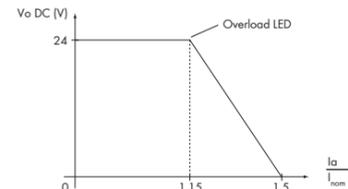
Fig. 4: Output characteristics
