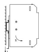
Fig. 2b: Disassembly
