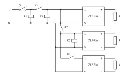
Fig. 3: Connecting power supply units in parallel
