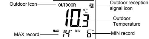
**Note:** The MIN/MAX outdoor temperature resolution is range -40°C to + 60°C with 1°C resolution.
