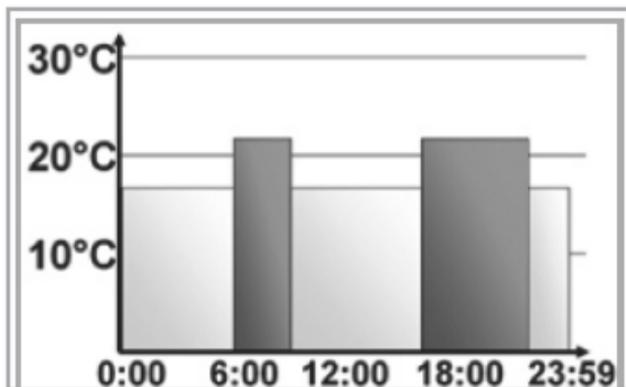
The display will show bars for those heating phases where the set temperature for the period is higher than the saved set-back temperature. In the example above, no bars are displayed for the phase between 0:00 and 6:00 o'clock. Only for the phases from 6:00 until 9:00 and 17:00 until 23:00 o'clock bars are shown in the display.
