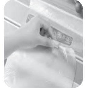
Make sure that you tighten the bag and the opening of the bag insert into the blade before you cut.
