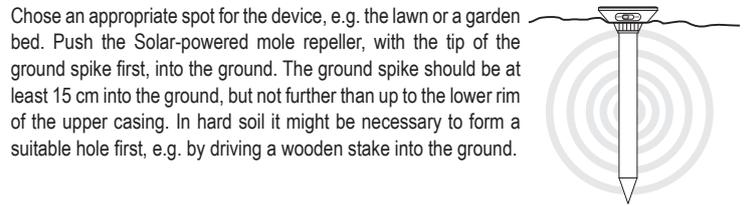
Choose an appropriate spot for the device, e.g. the lawn or a garden bed. Push the Solar-powered mole repeller, with the tip of the ground spike first, into the ground. The ground spike should be at least 15 cm into the ground, but not further than up to the lower rim of the upper casing. In hard soil it might be necessary to form a suitable hole first, e.g. by driving a wooden stake into the ground.
