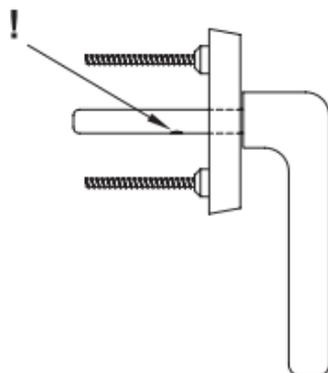
In order to push the window handle against the window rotary handle sensor without damaging it, all protrusions on the handle shaft must be removed.
