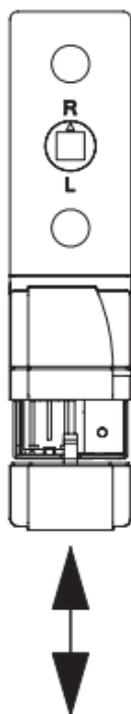
Push the battery compartment cover (arrow) downward and then remove it. Insert the two LR44 batteries provided with proper polarity according to the polarity markings into the battery compartment. The batteries are held in the battery compartment by the tension on the battery caused by the contacts. Note the flashing device LED when the batteries are inserted (see section "Behavior after inserting the batteries").
