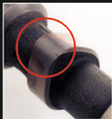
Visible cam wear.
