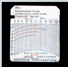
Compression diagram before engine flushing.
