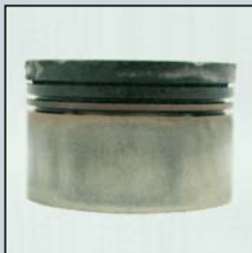
Deposits on the piston rings before flushing engine.
