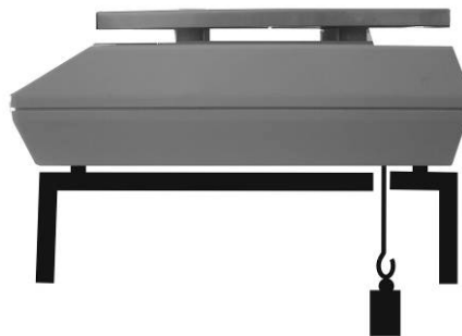
Fig. 1: Setup of balance for underfloor weighing
