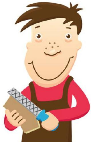
In order to saw empty spaces Sammy must first drill a hole in the sheet. Then, after having released the blade on one side, he pushes it through the hole, and secures it again. Now Sammy can cut out empty spaces. It's just that easy!
