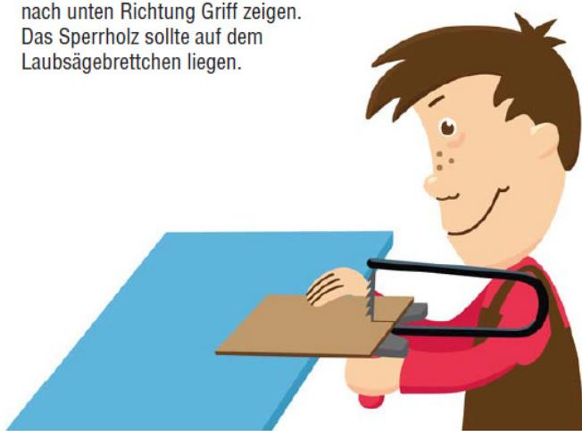
Now Sammy could saw, but he is holding the panel instead of securing it on the cutting table and the blade has been fixed with the teeth turned upwards, so that the wood is fraying.
