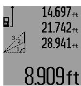
Upon completion of the last measurement, the result for the sought distance “**E**” is displayed in the result line **c**. The individual measured values are displayed in the measured-value lines **a**.
