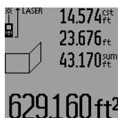
Now, measure length **B<sub>2</sub>** of the second wall. The individually measured value displayed in the centre measured-value line **a** is added to the length **B<sub>1</sub>**. The sum of both lengths ("sum", displayed in the bottom measured-value line **a**) is multiplied with the stored height **A**. The total surface value is displayed in the result line **c**.
