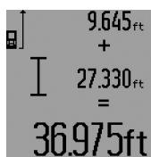
To call up the sum of both measurements, press the result button 5. The calculation is indicated in the measured-value lines a, and the sum in the result line c.
