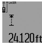
The current measured value is displayed in the result line **c**.
