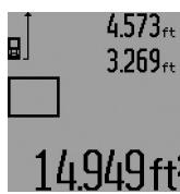
Upon completion of the second measurement, the surface is automatically calculated and displayed in the result line **c**. The individual measured values are displayed in the measured-value lines **a**.
