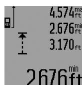
Depending on the set mode, the minimum or maximum value is displayed in the result line **c**. It is always overwritten, when the current length measurement value is less than the present minimal
