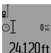
Then press the measuring button **7** to switch the laser beam on and aim at the target point. Press the measuring button **7** again to actuate the measurement. The measurement takes place after the set time period. The measured value is displayed in the result line **c**.
