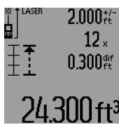
The mark-out value 2,0 ft is contained 12 times in a total distance of 24,3 ft. Additionally, the total distance contains a rest of 0,3 ft. Reduce the distance between the measuring tool and the starting point by 0,3 ft difference, and then mark off the length.
