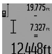
To subtract measuring values, press minus button **12**; For confirmation, “**-**” is indicated on the display. The further procedure is analog to “Adding Measured Values”.
