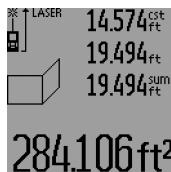
Afterwards, measure length **B<sub>1</sub>** of the first wall. The surface is automatically calculated and displayed in the result line **c**. The length measurement value is displayed in the centre measured-value line **a**. The laser remains switched on.
