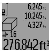
To recall the stored measurements, press button 15. The result of the last measurement is indicated on the display, along with the indicator for the measured-value list d as well as a counter for the numbering of the displayed measurements.
