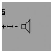
To switch the audio signal on and off, press the function-mode button **3** until the “audio-signal adjustment” indication appears on the display. Select the required setting by pressing the plus button **6** or the minus button **12**.
