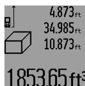
Upon completion of the third measurement, the volume is automatically calculated and displayed in the result line **c**. The individual measured values are displayed in the measured-value lines **a**.
