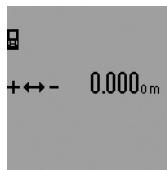
To change the unit of measure, press the function-mode button **3** until the "change unit of measure" indication appears on the display. Select the required unit of measure by pressing the plus button **6** or the minus button **12**.
