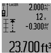
For a total distance of 23,7 ft, 0,3 ft are missing for the mark-out value 2,0 ft to be contained 12 times. Increase the distance between the measuring tool and the starting point by 0,3 ft difference, and then mark off the length.
