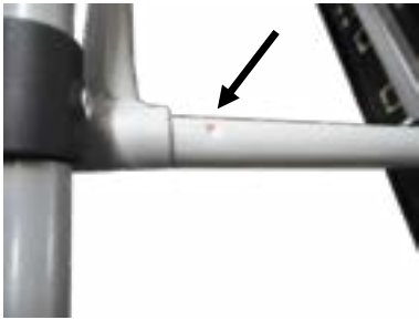
Figure 9: Marks on the lamp mount
