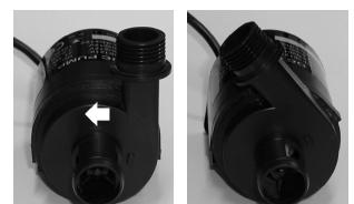
5. Take off the pump cover and pull the impeller with its bearing shaft out of the pump.
