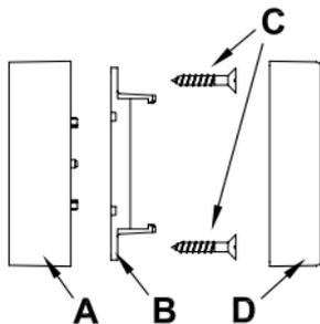
Then push the cover (D) of the magnets until latching on the magnet holder.
