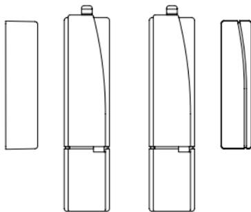
The installation surfaces of the two units (A and B) should match! This is achieved by inserting one or more of the provided spacer-pieces under the magnets (screw-mount only).
