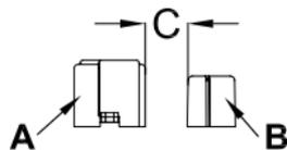
When "closed", the space C of the two units should not exceed 8 mm.
