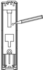
To actuate teach mode on the shutter contact, press the teach button with a pointed object. The device LED flashes orange.
