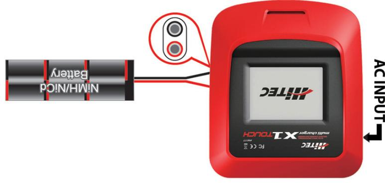
Connecting a battery directly to the charger to see the total voltage of a pack.
