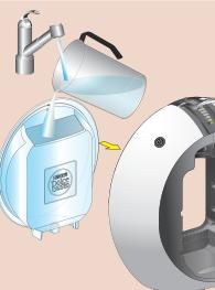
**EN** Check if there is water in the water tank. If not, refill and press „Start“ button again.
