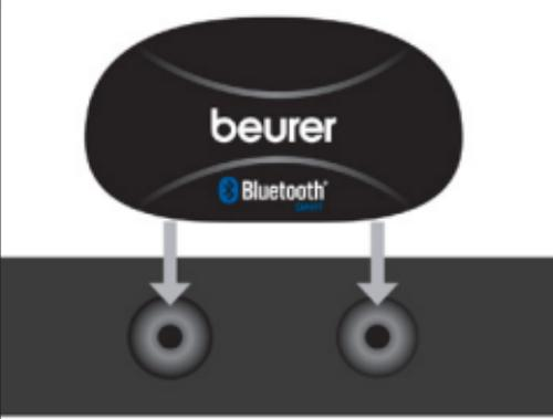
A diagram showing a black oval transmitter unit with the 'beurer' logo and a 'Bluetooth' symbol. Two grey arrows point downwards from the unit to two circular poppers on a dark grey chest strap. |
