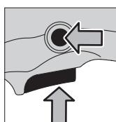
Press the lock-on button **3** to lock the pressed on/off switch **2**.
