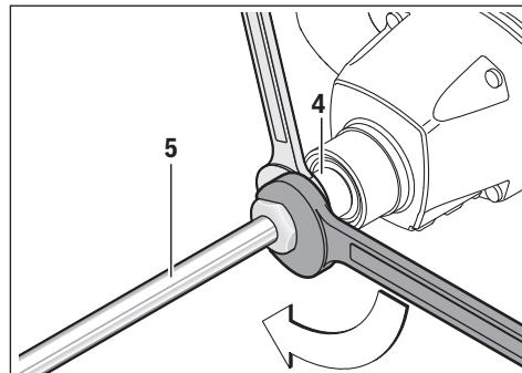
Screw the stirrer paddle 5 into the drive spindle 4. To do so, hold the drive spindle 4 using an open-ended spanner (GRW 12 E: width across flats 22 mm, GRW 18-2 E: width
