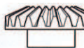
BA17 ×2 ベベルギヤ (大) Large bevel gear Kegelrad groß Grand pignon conique 51008
