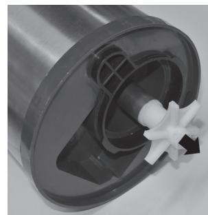
After this, you can remove the impeller (black arrow in the right image). As you are doing this, you have to overcome certain resistance due to magnetic force before the impeller can be removed.
