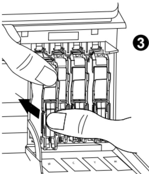
When the cartridge is empty, push the lever (A) up and pull the tab (B) to remove the cartridge from the printer.
