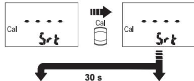
Push the button "CAL". Now one, two, three and then four dashes are shown in sequence. After approx. 30 seconds elapse, the status is displayed.
