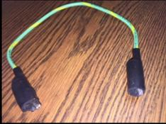
**2- Use an insulated clip lead jumper (~30cm) as shown.**
