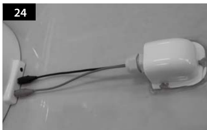
24 Connect black cable to the controller(middle) and grey cable to the receiver(Left).
