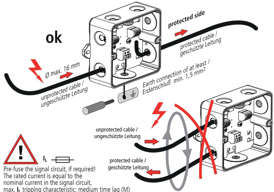
Pre-fuse the signal circuit, if required!
