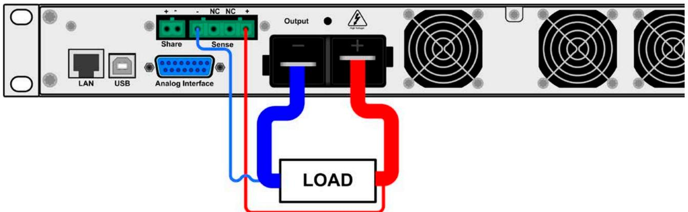
Figure 7 - Example for remote sensing wiring
