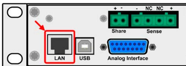
2. TCP/IP access via a freely selectable port (except 80 and other reserved ports). The standard port for this device is 5025, default IP is 192.168.0.2. Via TCP/IP and this port, communication to the device can be established in most of the common programming languages.
