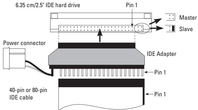
→ The IDE adapter contains no electronics assembly and simply converts differently shaped connectors and facilitates the voltage/current supply to the small 6.35 cm/2.5" hard disk (5 V/DC via PC adapter).
