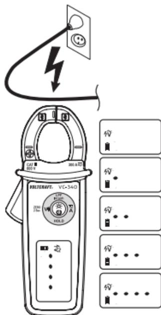
➔ The highly sensitive NCV sensor may also cause a voltage recognition at static charge. This is normal and not a malfunction.
