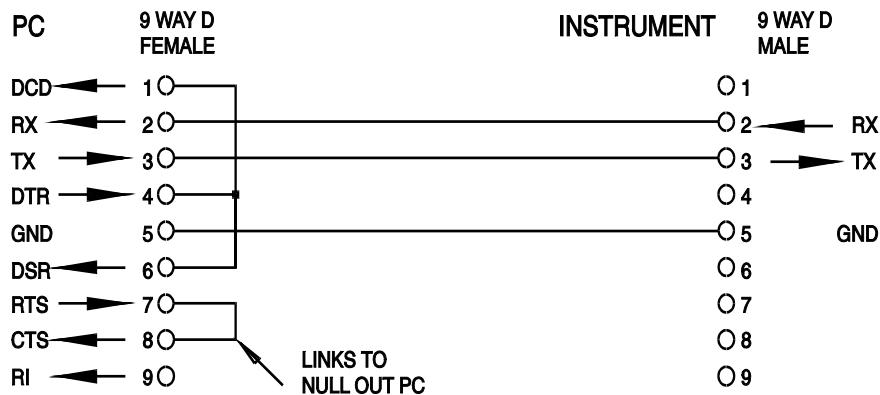
Baud rate is set as described above; the other interface parameters are fixed as follows:
