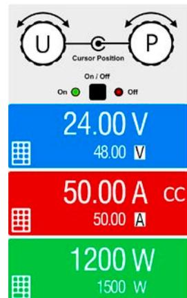
Depending on the selection the right rotary knob will be assigned different setting values, the left knob is always assigned to the voltage.
