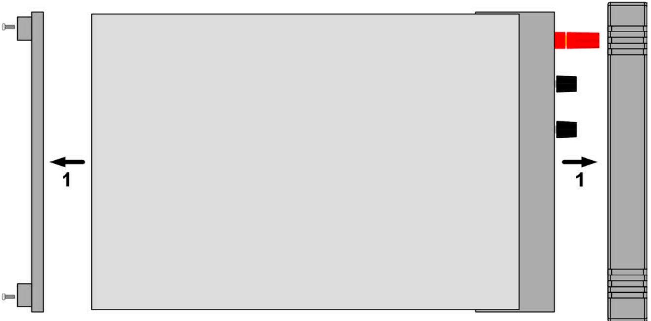
Figure 8 - Removal of the front and rear frame
