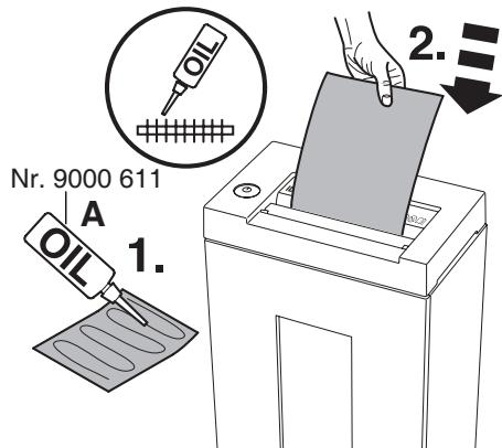
If the sheet capacity reduces or after the shred bin is emptied oil the shredding mechanism! (see picture)
