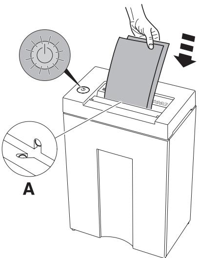
Feed the paper into the centre of the feed opening? (photo cell) (A)
