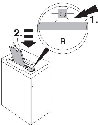
Is the rocker switch pressed? The green light rocker switch is ON? (1.).
