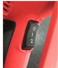
**WARNING:** The unit 1 minute lowest temperature (50 ° - Level 1) leave to cool in operation before the device is switched off completely.
