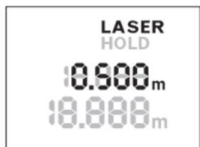
Press the “HOLD” button **2** once more to switch the laser on again. The **LASER** indicator flashes on the display. The previous measuring value is displayed in the top line. The continuously updated/current measuring value is displayed in the bottom line.
