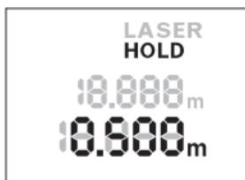
Press the "HOLD" button **2** to stop the measuring procedure. The laser beam is switched off and the **HOLD** indication appears on the display. The current measuring value is still displayed in the bottom line of the display, but is no longer continuously updated.
