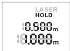
Press the “HOLD” button **2** once more to stop the measuring procedure again. The laser beam is switched off and the **HOLD** indication appears on the display. The previous measuring value is displayed in the top line. The current measuring value is displayed in the bottom line, but is no longer continuously updated.
