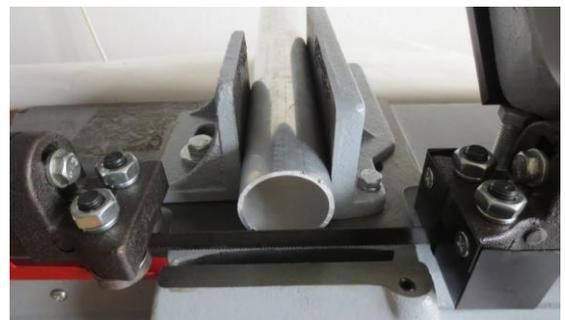
**CAUTION:** Bevel cuts are resulting from not exactly vertical set saw blade guides and too much play between the lateral bearing rollers!
