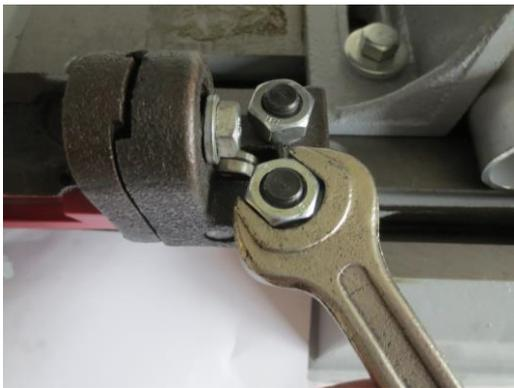
Slightly loosen the nuts on either side guide rollers with a wrench **SW17**.
