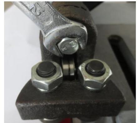
**NOTE:** Check the 90 ° bandsaw blade guide with an angle gauge or with a rectangular workpiece.
