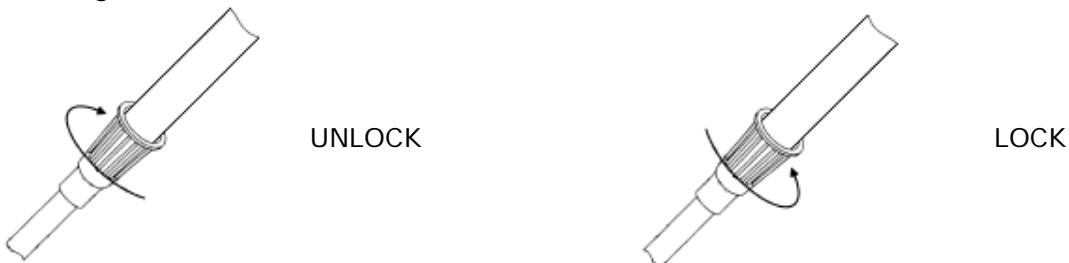
**Note:** the coils' wiring runs inside the stem. Do not force to avoid damage.
