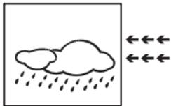
In the default setting of the weather station, the barometric pressure must drop by 4 hPa.
