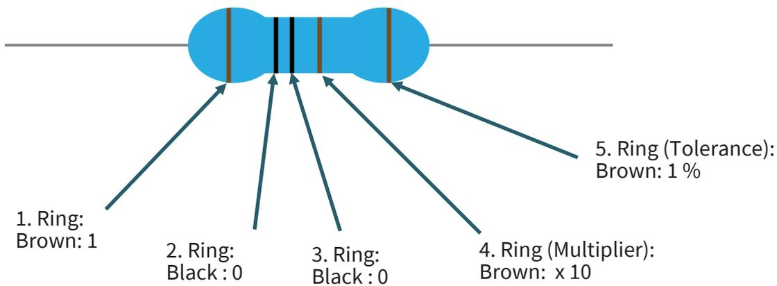
The first three rings give the first value of 100, which is calculated by means of the multiplier (x 10) to the resistance value of 1000  $\Omega$ . This can also be converted to 1 k $\Omega$ . So this has resistor a resistance value of 1 k $\Omega$  with a tolerance of 1 %.
