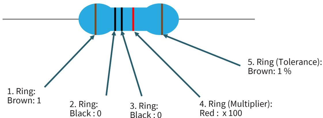
The first three rings result again in the first value of 100. By means of the multiplier of x 100 the resistance value of 10.000  $\Omega$  is obtained, which can be converted into 10 k $\Omega$ . Also this resistor has again a tolerance of 1 %.
