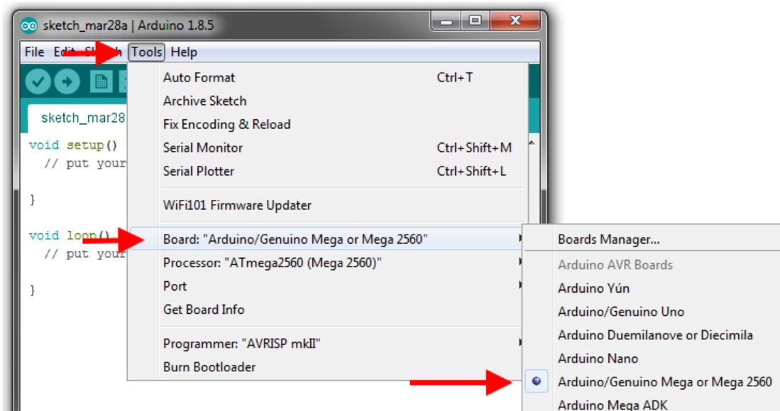
2. Under **Tools** → **Port** then select the port which is marked with **Arduino/Genuino Mega or Mega 2560**.
