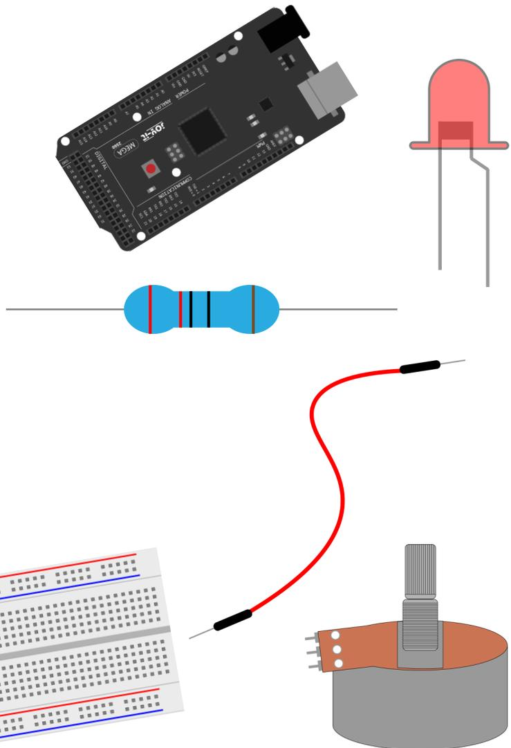
The input of the potentiometer is analog, so we connect it to the analog port. We connect the LED to the PWM port. A other PWM signal can regulate the brightness of the LED.
