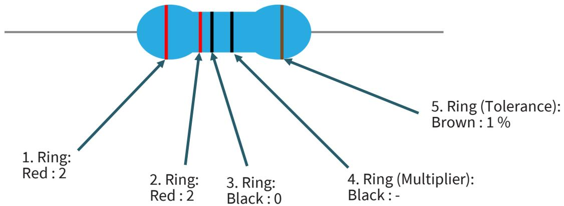
Due to the fact that the multiplier has no value, the resistance can be determined on 220  $\Omega$  with a tolerance of 1%, which this resistance can vary.
