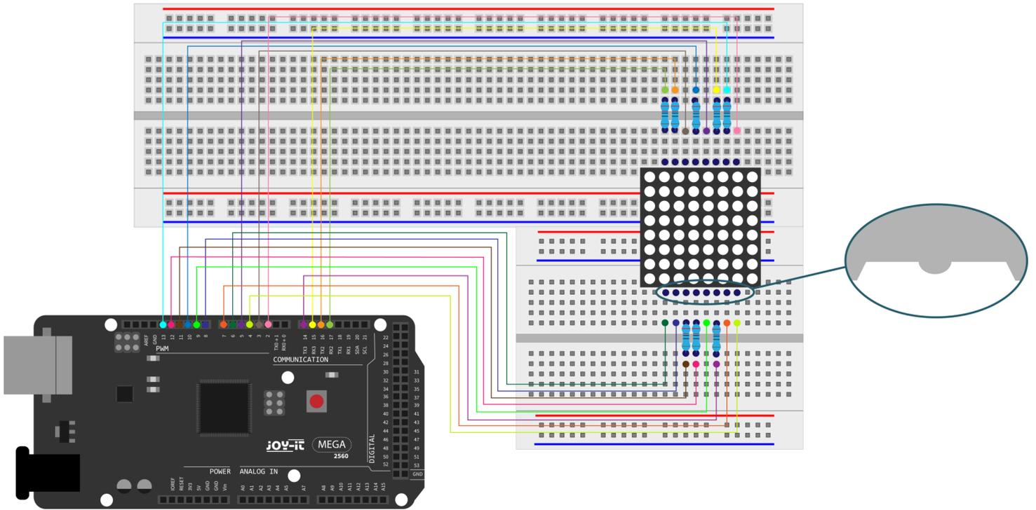
Make sure that the LED matrix is connected properly. Under the matrix there is a bulge (picture) where you can compare the position of your matrix with the matrix on the picture.
