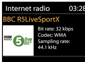
If you are already listening to an Internet Radio station, you can press **BACK** or **◀** on the remote control to quickly return to the last visited branch of the menu tree, rather than press and hold **MENU** to go to the first menu of Internet Radio mode. Press **▶||** to pause playing. Press again to play the station.
