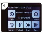
The LCD panel displays the status notification < filament changing >. The 3D printer is now ready for the filament feed-in.
