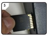
• Insert the SD card with the label side facing downwards.
