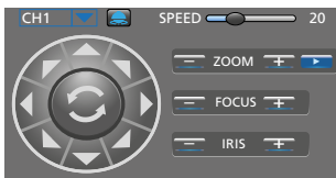
Fig. 7-20 Window for PTZ control
