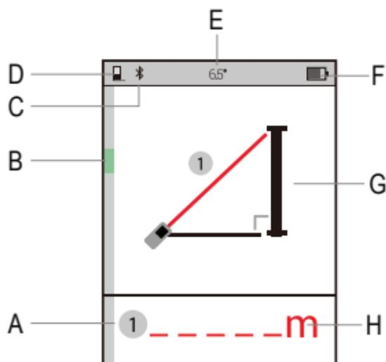
→ Example: Indirect measurement with two reference points
